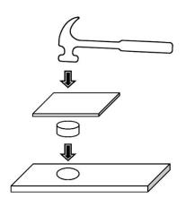
NOTE: You will have to destroy the plugs to disassemble the base. We have supplied enough plugs to disassemble and reassemble once, although you may wish to move the base without taking it apart to avoid this issue.
